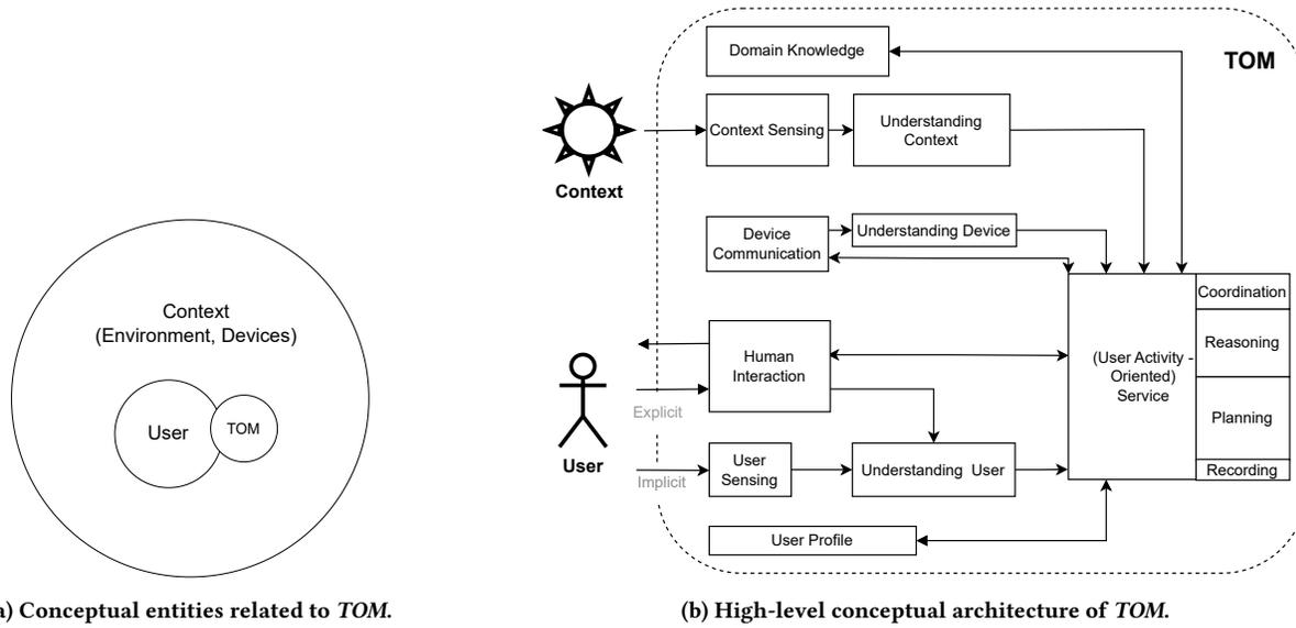
**Figure 1: Conceptual entities and high-level modules associated with TOM. Arrow directions represent the communication (e.g., data/interaction) flow.**
