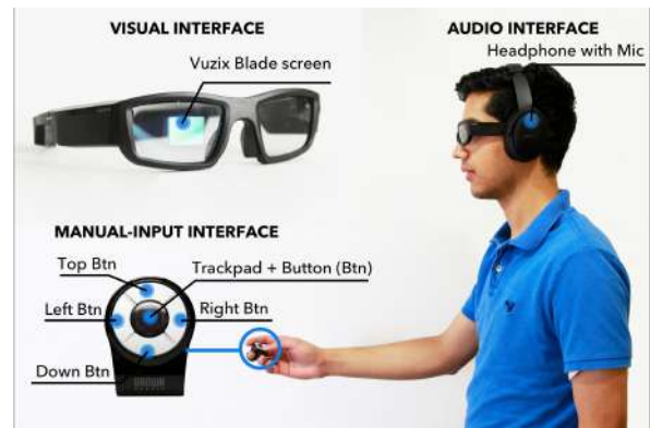
Figure 2: Apparatus showing all three interfaces.
